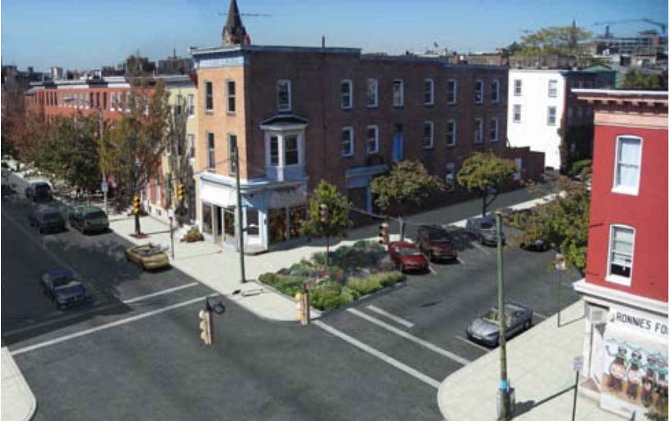
Phase 2: Stormwater runoff collection bumpouts on angled parking side of N/S streets
