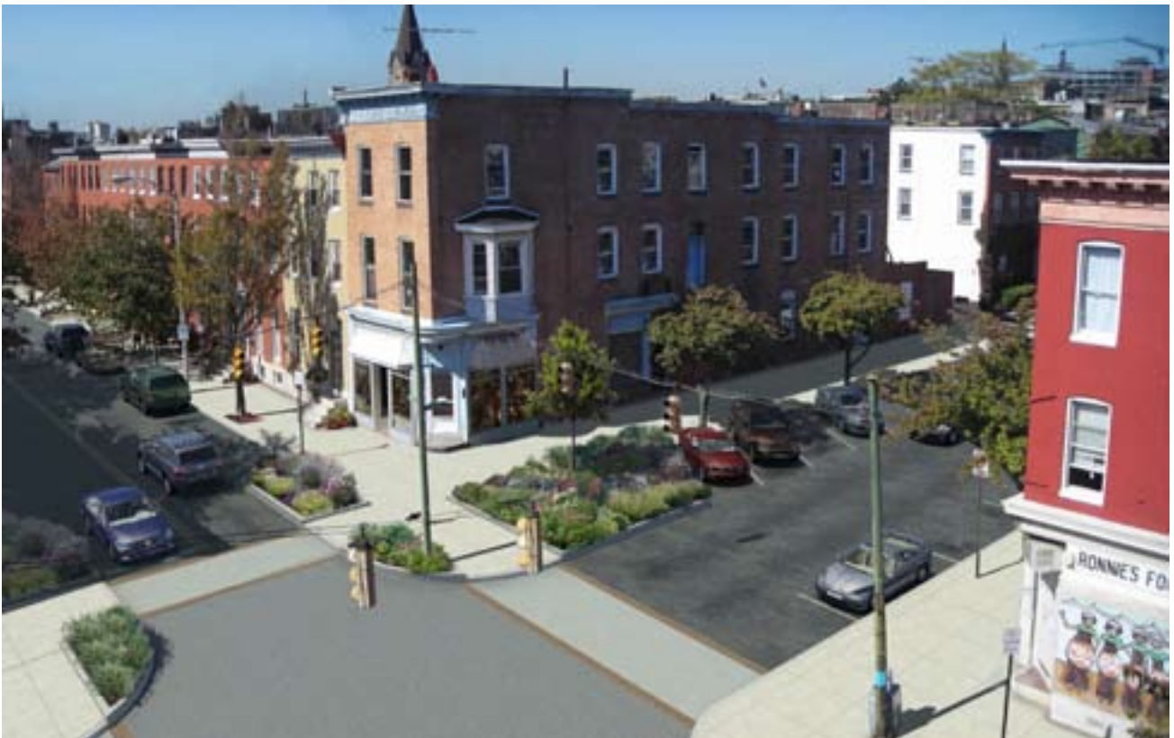
Phase 3: Bumpouts and textured crosswalks along E/W streets as traffic calming devices
