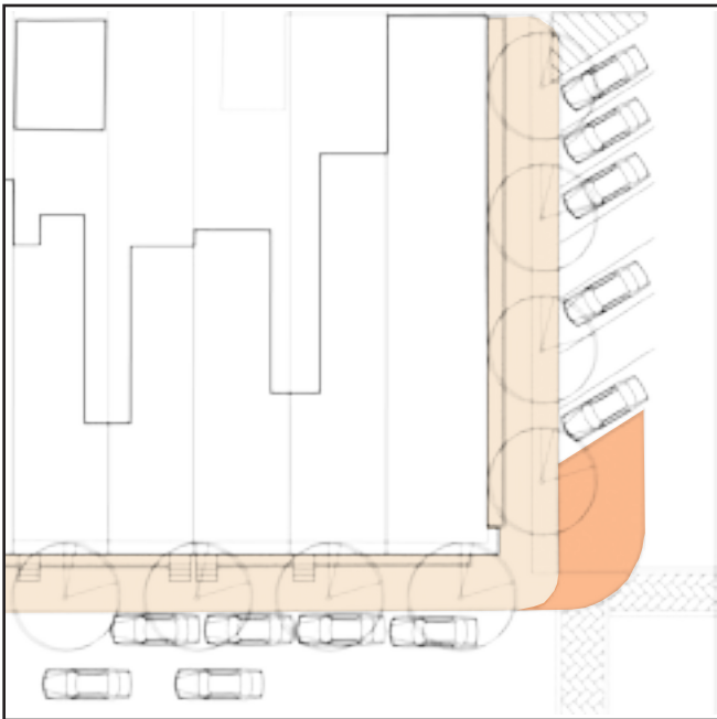
Proposed angled parking (with N/S bumpout) - allows for the creation of stormwater curb extension to help manage runoff - reduces pedestrian crosswalk distance - traffic calming - does lose 1-2 parking spaces - plantings in bumpout enhance character of streetscape
